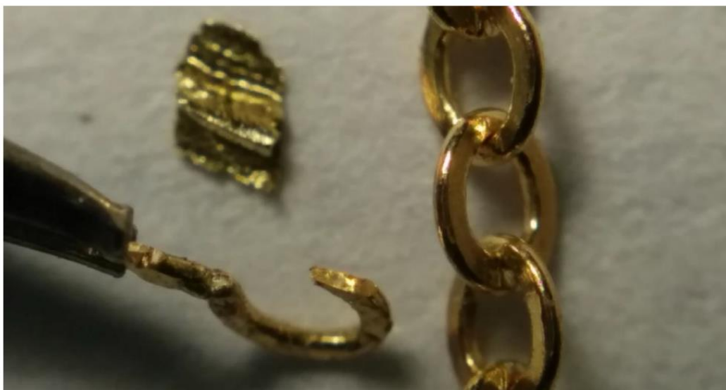
Figure 1: Check for Gold Plating. A single link was cut to check for possible differences between the core and exterior of the sample. Color is consistent throughout the sample.
